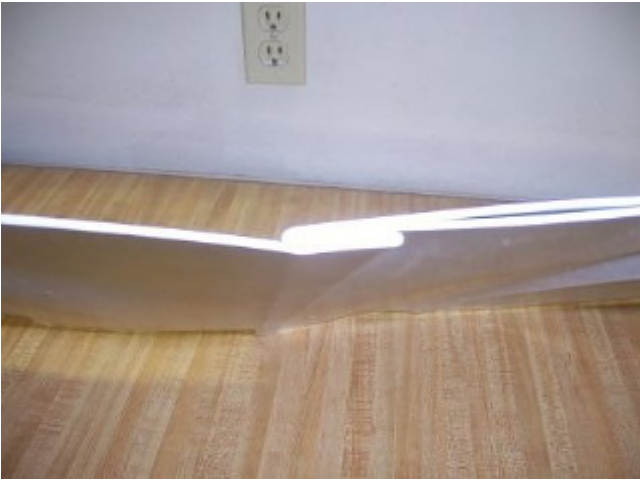
The 2 pieces of siding join like so.
